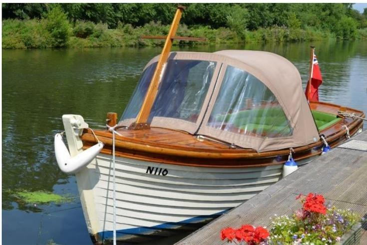
Meanderer was originally built in 1952 for use as a working harbour launch and spent most of her life in and around the Norfolk coast and the Broads. Her construction comprises of a clinker-built wooden hull and superstructure and has an inboard Vetus 3-cylinder diesel engine.
